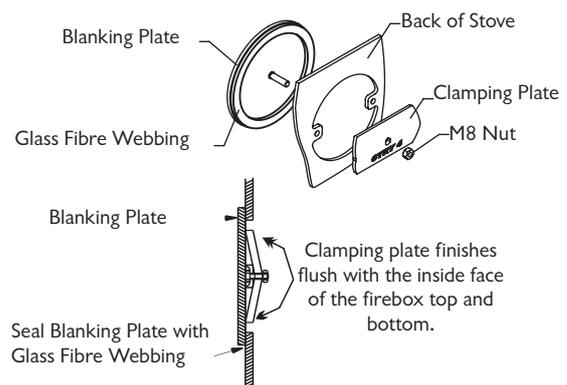
webbing fitted to its sealing face, and fitted to the rear flue outlet.
