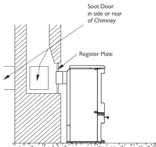
**Fig.8. Horizontal register plate with rear flue connection**
